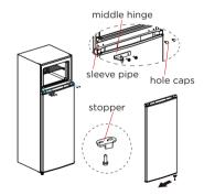
**8.** Assemble the stopper of the freezer door on the other side.
