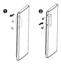
**Step 2:** Install the door handle to the door and fasten it with screws
